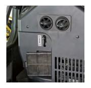
The air filters are easily accessible for an improved maintenance.
