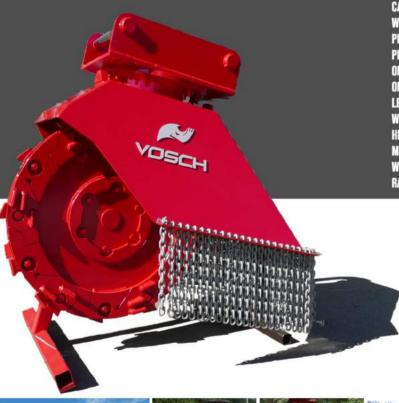
S6720 S6900 S6900 HD 13-25 18-30 **CARRIER (TONS)** 7-12 **WEIGHT (KG)** 480 640 680 PRESSURE MAX (BAR) 350 350 PRESSURE ROTATE (BAR)\* 190-210 190-210 190-210 OIL FLOW MAX (L/MIN) 100-120 120-140 275-325 OIL ROTATE (L/MIN)\* 25 25 25 LENGTH (MM) 1200 1450 1450 WIDTH (MM) 900 1050 1150 **HEIGHT EX ADAPTER (MM)** 900 1100 1110 MOTOR DISPL. (CCM) 80 110 250 WHEEL DIA (MM) 720 900 900 RATES (RPM) 1300-1500 1100-1300 1100-1300
